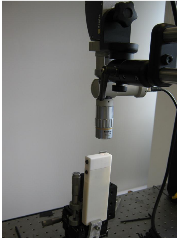
Figure 4-7: Braille pin displacement validation using a laser vibrometer.
