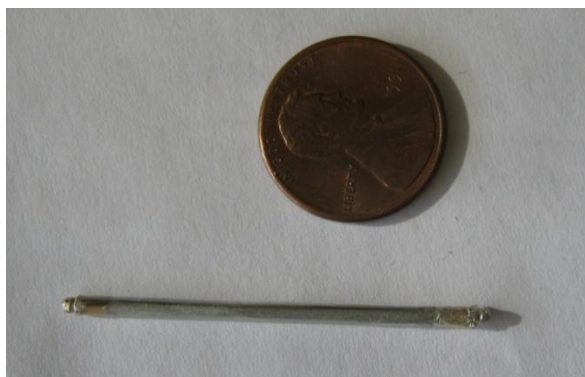
Figure 2-3: Photograph of a finished actuator made with the actuator rolling machine
